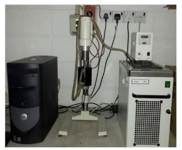
Figure 2: Controlled-stress rheometer
